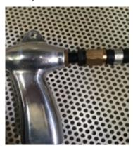
The adjustment is a "trial and error" process. The adjustment allows for the sandblaster to work as efficiently as possible based on particular needs and set up. Once the optimal position has been found for the gun make sure that the bronze locknut is re-tightened.
